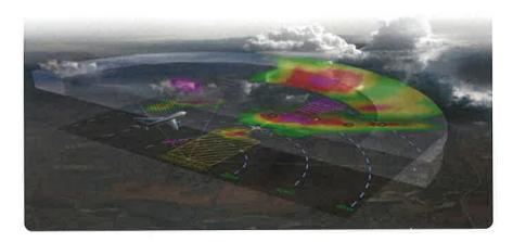
The RDR-7000 scans all the weather in front of the aircraft out to 320NM and from the surface to 60,000 feet, filling a 3-dimensional buffer, and even maintains weather information that shows the weather as it passes behind the aircraft.
